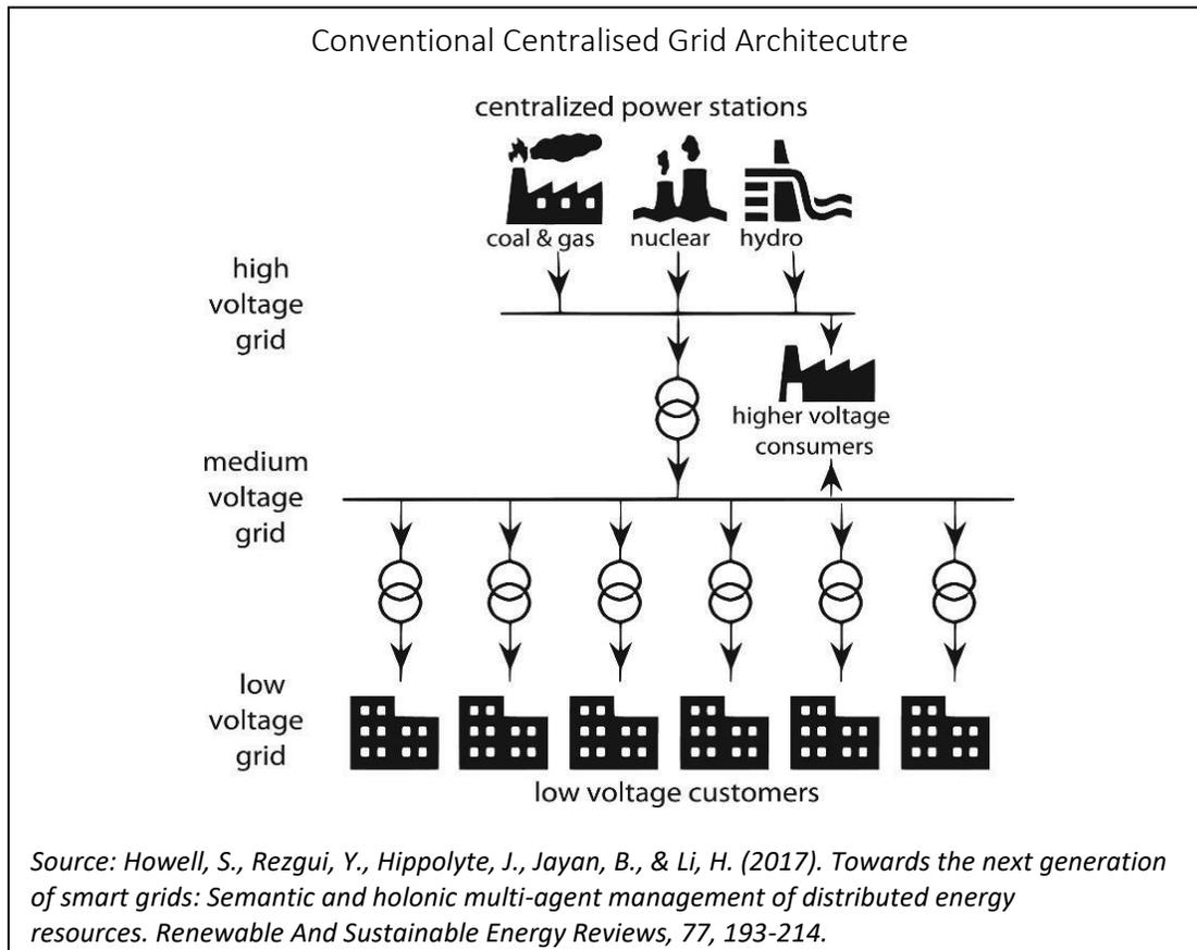
Figure 3: Schematic of Conventional Centralised Grid Architecture
