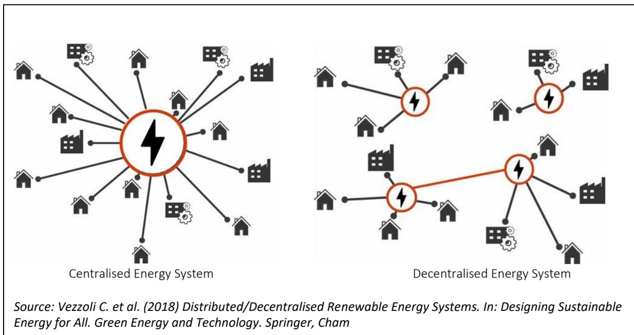
Figure 5: Schematics of Centralised and Decentralised Energy Systems
